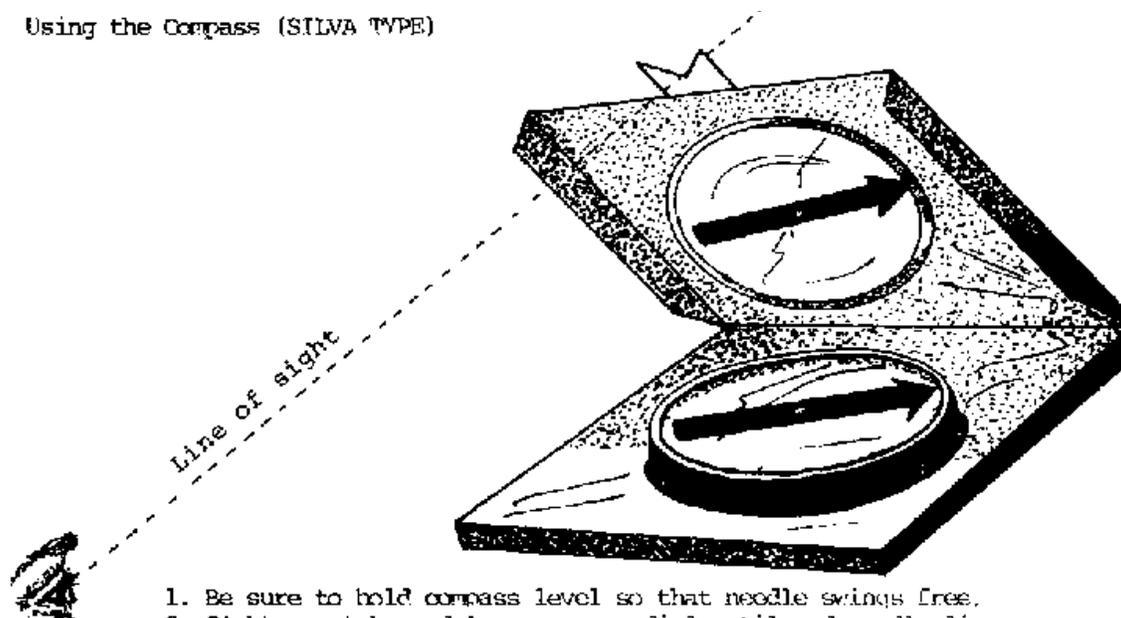
1. Be sure to hold compass level so that needle swings free.
