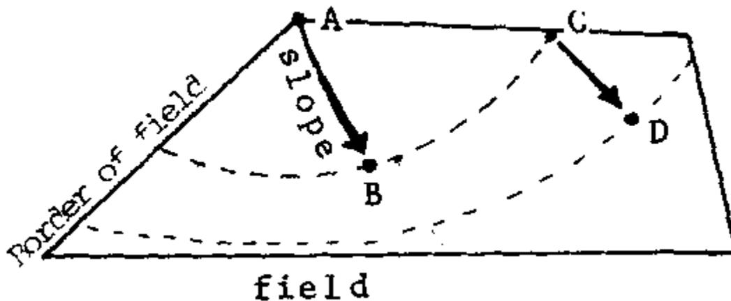
Using the rustic instruments, points can be Marked every 10 or 15 meters. The points are marked by driving a stake into the ground. Using a surveyor, level points can be placed every 30 - 35 meters. A helpful way to measure these distances is to tie a light weight rope between the sighting instrument and the sight rod.
