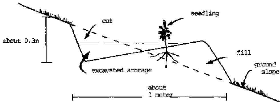
Gradonis Spacing - is determined by the desired tree spacing usually 2 x 2 or 3 x 3 meters. The closer spacing is recommended on the critical eroding areas to obtain a quicker crown closure and litter (mulch deposit on the forest floor). The trees can be thinned as needed to maintain plant vigor. The thinnings can be utilized for fuel or other uses.
