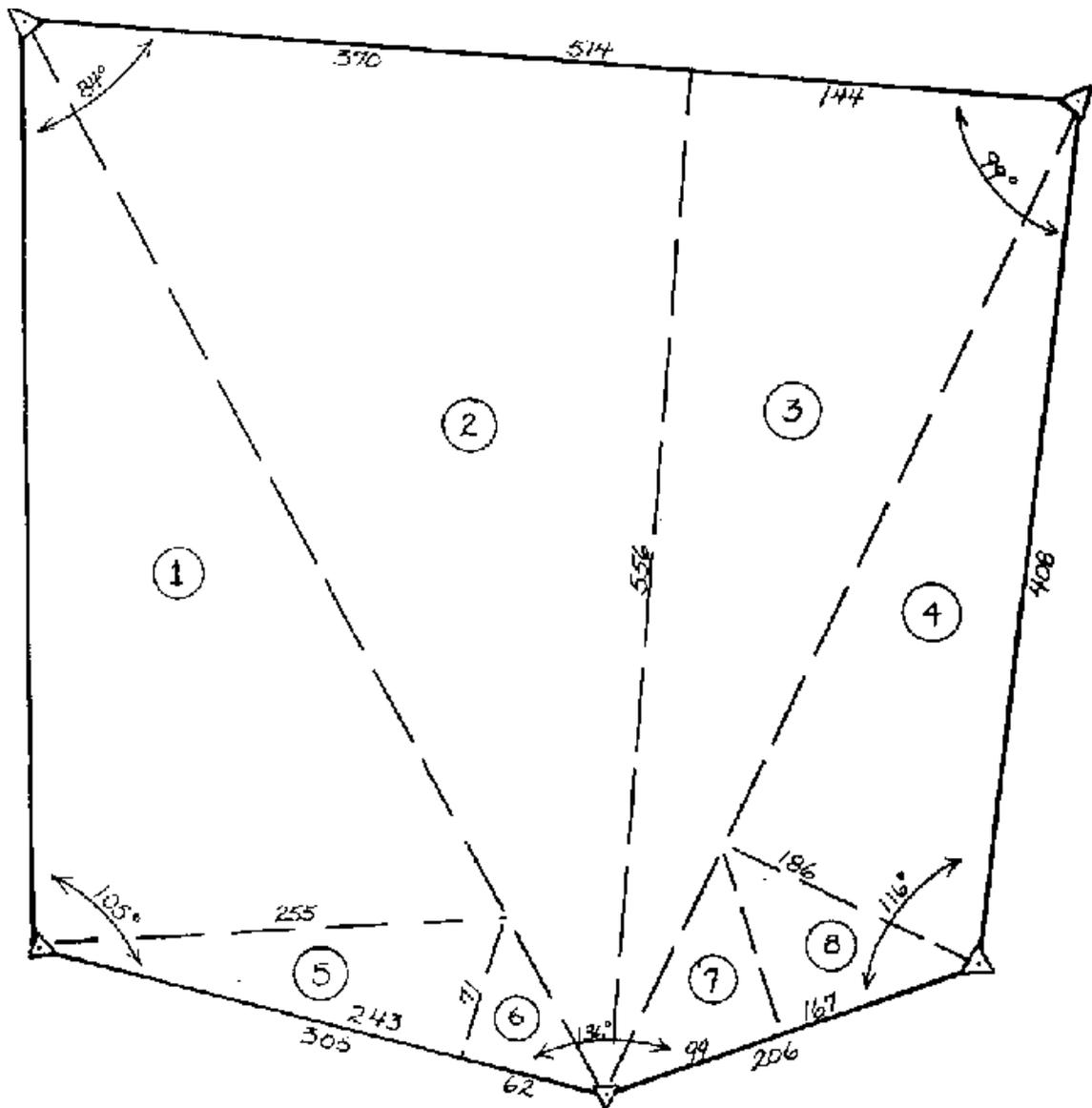
Draw traversed figure to scale on graph paper. Break into triangles and scale off distances.
