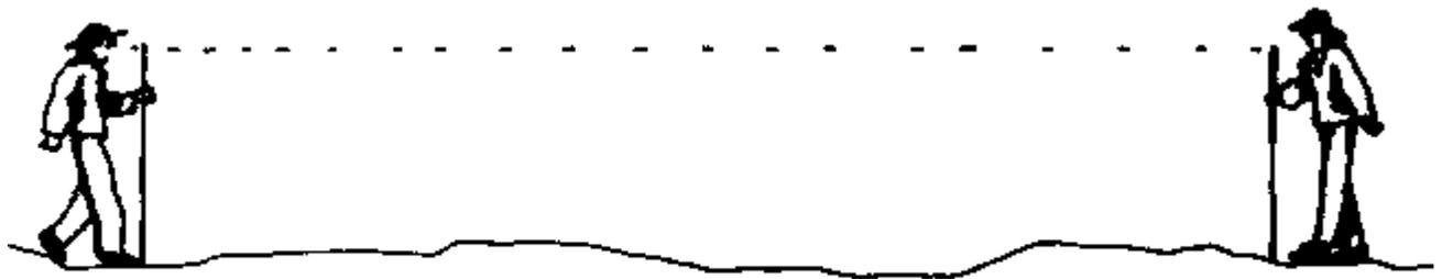
You have the man move up or down the slope until you see your mark through the sight. Then he puts a stake in that spot, and then its on to the next mark. Fairly soon, you would have stakes all along the contour of the slope for that particular terrace (curvas).
