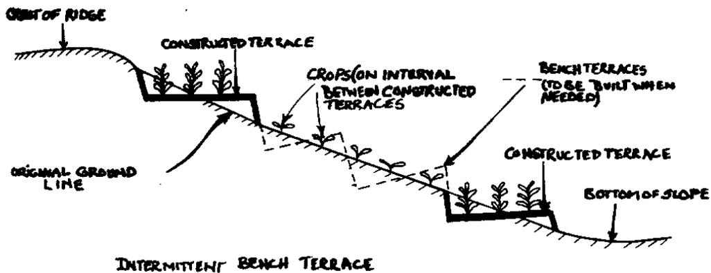
Bench Terraces should be no longer than 10 meters - runoff from longer terraces is difficult to manage. The horizontal grade of toe-drain is 1 percent to safe outlet (waterway).
